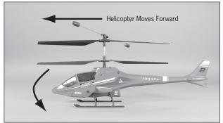
Pulling the stick backward will pitch the nose of the helicopter upward, allowing the helicopter to be flown backward.
