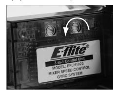
Note: You must always power down the 3-in-1 unit before making adjustments to the proportional mix trimmer pot. Any changes made to the trimmer pot will not take effect until the 3-in-1 unit is re-initialized and re-armed.
