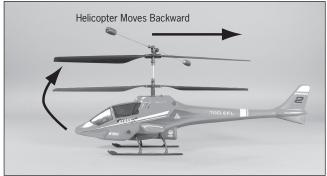
The elevator trim can be used to help keep the helicopter from drifting forward or backward when in hover with no elevator stick input. For example, if the helicopter drifts forward when in hover, pull the elevator trim downward until the helicopter hovers as level as possible with no forward drifting.
