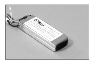
The battery can be installed through the opening in the rear of the body. Be sure to install the end of the battery with the loop material first. If you have installed the loop material on the end of the battery with the wire leads, be sure that the wire leads are oriented to the left side of the model so that they can pass by the stop. Slide the battery into the support frame until the hook and loop material makes contact.
