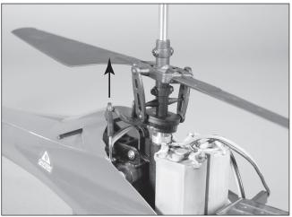
When the stick is pushed to the right, the forward servo should pull the swashplate downward.
