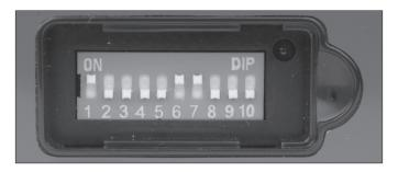
If the controls still do not respond properly after ensuring that the servo reversing dip switch positions are correct, you may also check the servo connections on the receiver side of the 3-in-1 unit. These should be positioned as follows (when viewing the helicopter from behind):
