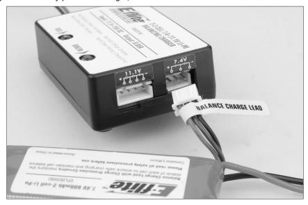
When the battery is properly connected and charging normally, the red and green LED indicators will glow solid. Once the battery has been fully charged, the green LED will go out, leaving just the red LED glowing solid. The battery can now be removed from the charger and installed into the Blade CX2 for flight.
