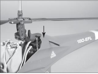
Position the helicopter to view it from the right-hand side. Move the aileron control stick on the transmitter left and right to check aileron roll control. When the stick is pushed to the left, the forward servo should push the swashplate upward.
