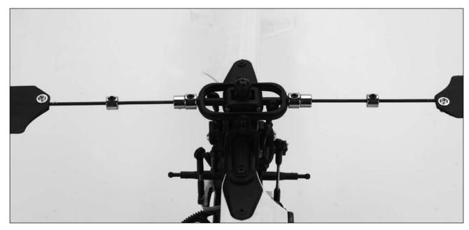
Dampening of the rotor head (main rotor blades) can also be adjusted in order to fine-tune the cyclic response of your model. In general, stiffer dampening will result in quicker cyclic response. The dampening of your Blade SR has been set to provide good stability right out of the box, and we suggest that you make your first flights with this amount of dampening before making any changes.
