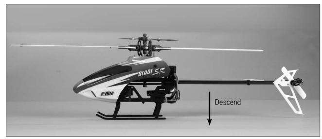
After lifting the model off the ground you can balance the throttle/pitch by carefully moving the left-hand stick up and down so the model will hold a stationary hover without climbing or descending.
