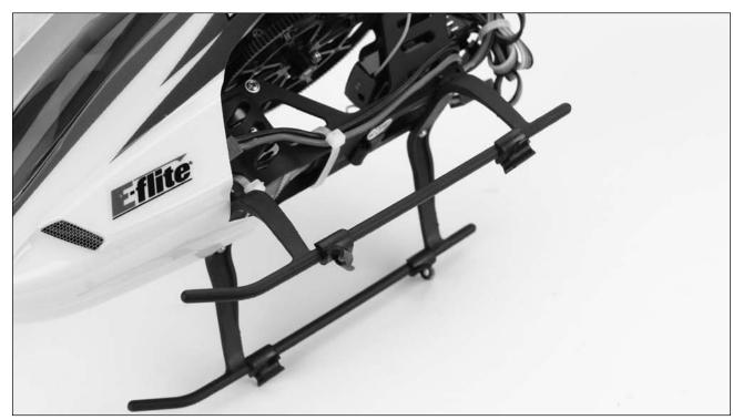
• Carefully pass each of the rods through the holes in the attachments on the landing skids and into the of the parts.
