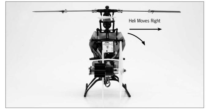
Use the aileron trim to help keep the helicopter from drifting left or right when in hover with no aileron stick input. For example, if the helicopter drifts to the right when in hover, add left aileron trim until the helicopter hovers as level as possible with no drifting to the right.
