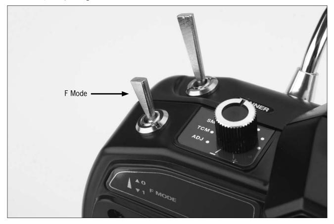
Toggling the flight mode switch toward the rear of the transmitter (position 0) puts the transmitter/helicopter in normal flight mode. In this flight mode, the throttle curve is programmed from 0% to 100%. This is the preferred flight mode for general hovering.
