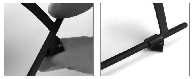
• After installing all four attachments, locate the four training gear rods and rod mounting base. Note that the rod mounting base has a "coned" shape to it. The "pointed" side of the base will face upward toward the bottom of the helicopter when properly installed. The base also has two different angles where the gear rods attach. It is important to orient the base so that the large angle is facing forward and backward.
