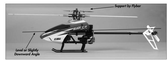
**Note:** Before each flight ALWAYS turn the transmitter on before connecting the flight battery to the 2-in-1 unit. After each flight, you should always disconnect the flight battery from the 2-in-1 unit before powering the transmitter off.
