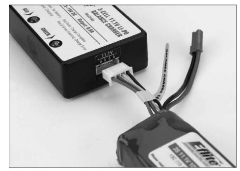
When the battery is properly connected and charging normally, the red and green LED indicators will glow solid. Once the battery has been fully charged, the green LED will go out, leaving just the red LED glowing solid. The battery can now be removed from the charger and installed into the Blade SR for flight.
