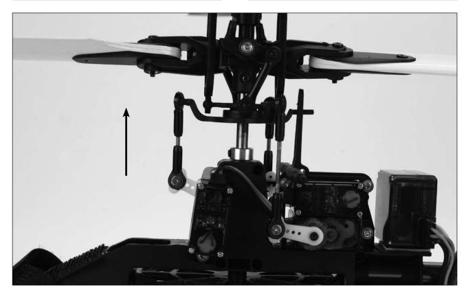
Again viewing the helicopter from the left or right side, move the right-hand stick forward and aft to check elevator pitch control. When the stick is pushed forward, the swashplate should also tilt forward.
