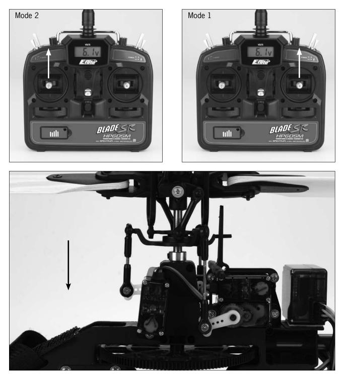
With the stick pulled back down, the swashplate should raise, decreasing the pitch of the main blades.
