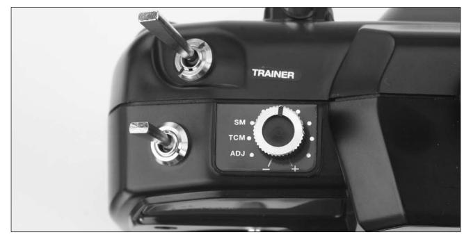
The SM TCM ADJ knob offers you the ability to adjust the main rotor head speed, and in turn the collective and cyclic control response of the model between the endpoints of the throttle curve in the stunt flight mode. Typically, a higher main rotor head speed will result in guicker collective and cyclic control response around middle stick.
