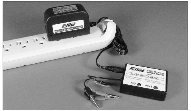
Input power for the charger can also be supplied from a small 12-volt gel cell or car battery.
