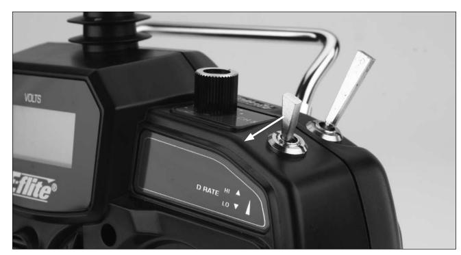
If the Blade SR is your first single-rotor and/or collective-pitch equipped helicopter model, we strongly recommend that you make your first flights with the dual rates set to low.
