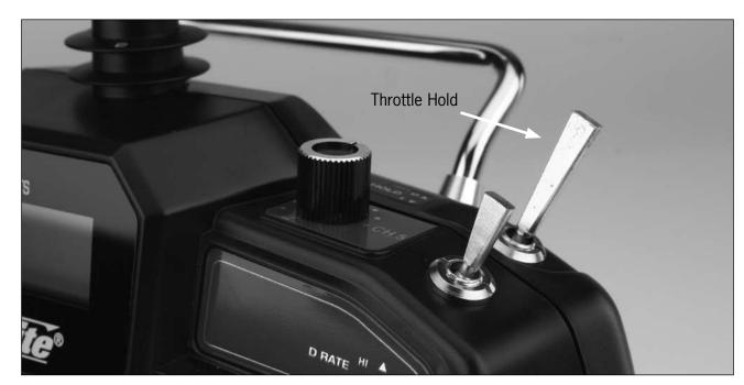
When the throttle hold switch is toggled toward the rear of the transmitter (position 0), throttle hold will be off. When throttle hold is off, the transmitter will be in the normal or stunt flight mode (depending on the position in which the F MODE switch is set).
