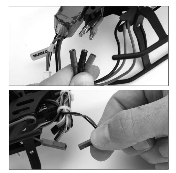
Turn the transmitter on first and lower the throttle stick and trim completely. Then, plug the battery into the battery lead of the 2-in-1 unit.
