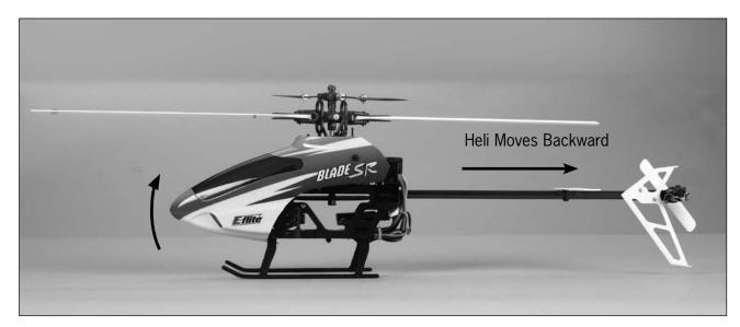
The elevator trim can be used to help keep the helicopter from drifting forward or backward when in hover with no elevator stick input. For example, if the helicopter drifts forward when in hover, pull the elevator trim downward until the helicopter hovers as level as possible with no forward drifting.
