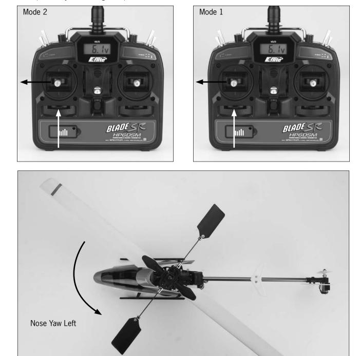
Moving the stick to the right will turn (yaw) the nose of the helicopter to the right about the axis of the main shaft. This is accomplished by increasing the speed of the tail rotor blade.
