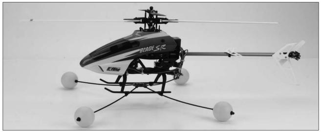
channels on the base. The rods will pass through the front holes of the forward attachments, and the back holes of the rear attachments. You may find it necessary to apply some light pressure to the rods, base and landing skids when installing all four rods in the base. This is typical; however, take care to not damage any
