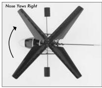
The rudder trim can be used to help keep the nose of the helicopter from rotating to the left or right when in hover with no rudder stick input. For example, if the nose of the helicopter drifts to the right when in hover, add left rudder trim (by pressing the left-hand rudder trim button) until the nose stays as close to straight as possible.
