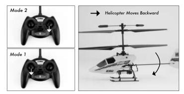
The elevator trim can be used to help keep the helicopter from drifting forward or backward when in hover with no elevator stick input. For example, if the helicopter drifts forward when in hover, add back/up elevator trim until the helicopter hovers as level as possible with no forward drifting.
