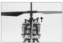
Move the aileron stick left and right to check aileron roll control. When the stick is pushed to the left, the left-hand servo (when viewing the helicopter from behind) should pull the swashplate downward.
