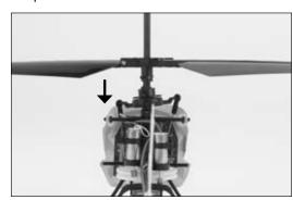
With the aileron stick pushed right, the left-hand servo should push the swashplate upward.
