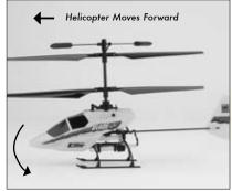
Pulling the stick backward will pitch the tail of the helicopter downward, allowing the helicopter to be flown backward.
