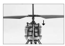
With the stick pulled back, the right-hand servo should push the swashplate upward.
