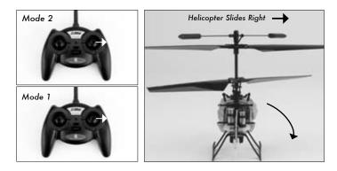
The aileron trim can be used to help keep the helicopter from drifting left or right when in hover with no aileron stick input. For example, if the helicopter drifts to the right when in hover, add left aileron trim until the helicopter hovers as level as possible with no drifting to the right.
