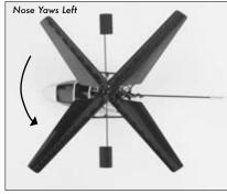
Moving the stick to the right will turn (yaw) the nose of the helicopter to the to the right about the axis of the main shaft. This is accomplished by increasing the speed of the upper main rotor blade while decreasing the speed of the lower main rotor blade.
